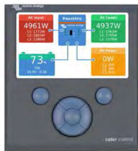
Color Control panel, showing a PV application
