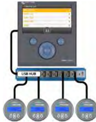
A maximum of four BMVs can be connected directly to the Color Control. Even more BMVs can be connected to a USB Hub for central monitoring.
