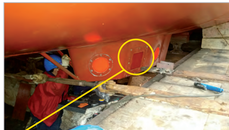
Installed looking to the port side of the vessel together with horizontal looking ES70 echosounders previously installed.
